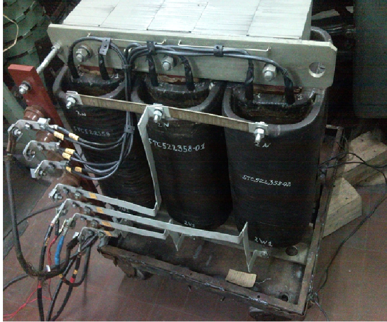
Figure 2. Three-phase transformer T-164 with the scheme and winding connection group Dyn7 for usage onboard of electric locomotive
